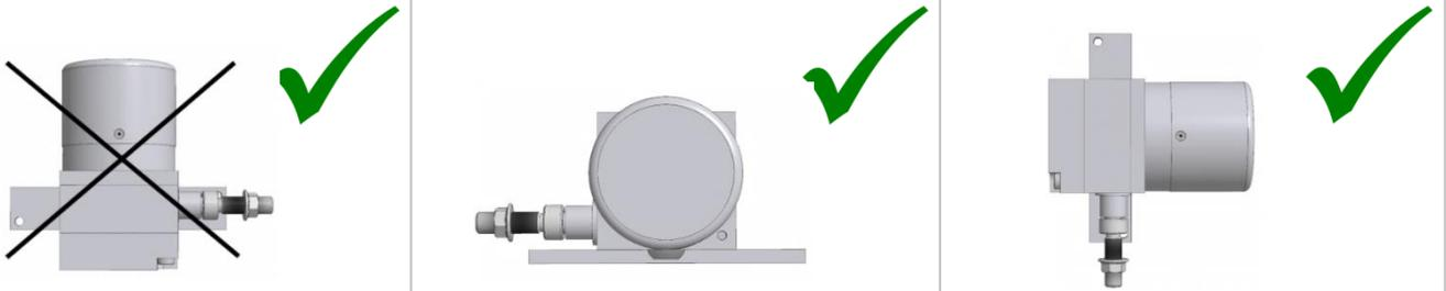
**3. If there is a trickle of water (like a rain), the wire outlet must not be a drip of water upstream. If needed please use guide rollers.**
