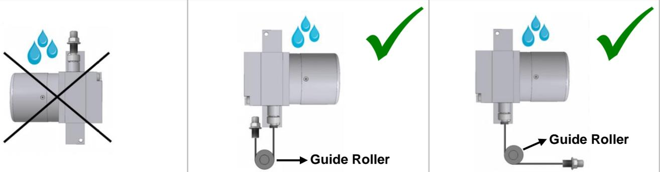
**4. The wire should not be pulled in angular. If needed, please use guide rollers.**
