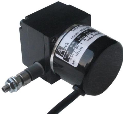
AWE 110 wire encoders convert linear motion into incremental digital pulses. Different stroke lengths from 300 mm to 1250 mm are available. Optionally other stroke lengths, resolutions, cable lengths and socket connectors can be requested.
