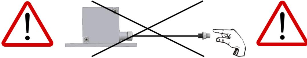
**2. The wire encoder must be mounted vertically in position, not be horizontally.**
